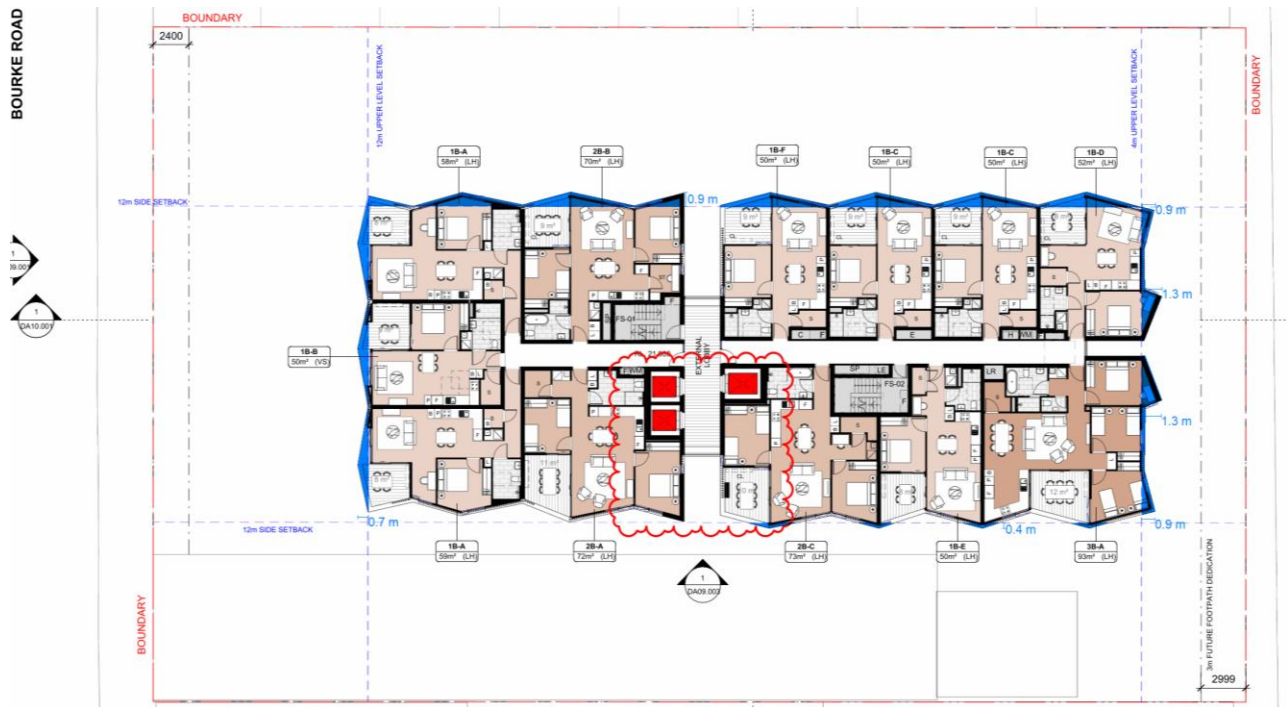
Figure 22: Point encroachments into the ADG Part 2F building separation distances - typical floor plate 4-14
